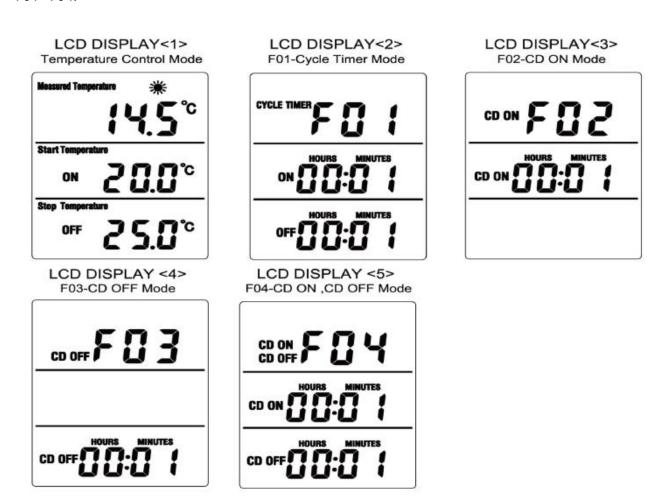
F01 Cyclic Timing Mode: Cycle by start time (ON) and stop time (OFF).
