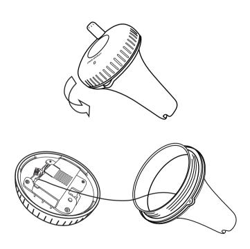
Remove the battery cover, install 2 AAA batteries, put the cover back.
