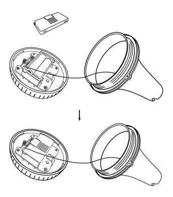
Make sure the silicone waterproof ring is well placed, then close and tighten the lid of the pool thermometer.
