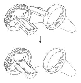
Make sure the silicone waterproof ring is well placed, then close and tighten the lid of the pool thermometer.
