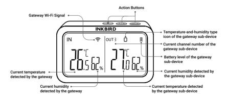
The INKBIRD Wi-Fi Gateway is specially built for some INKBIRD Bluetooth/Wireless devices, offers mobile network connectivity, and ensures that all synchronized devices can be managed with the INKBIRD app.
